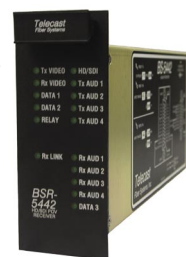
Modules are available as "throw down" units or may be rack mounted in the popular Viper II frame.
