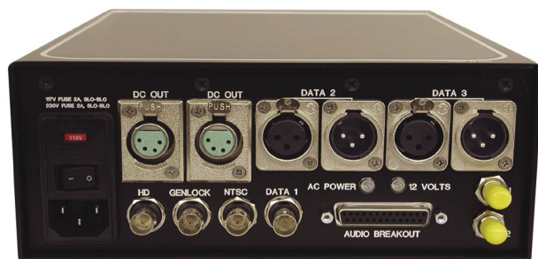
Ruggedized CA5442X custom package, designed for Fletcher Chicago, brings AC power input, DC output and a connector set specially adapted for HD sports production
